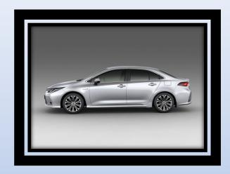
MODEL CODE MZEA11L-GEXDBV ENGINE: M15A-FKS, 1.5L, 3-CYLINDERS MAX OUTPUT: 119 HP / 6500-6600 RPM MAX TORQUE: 148 NM / 4600-5000 RPM
